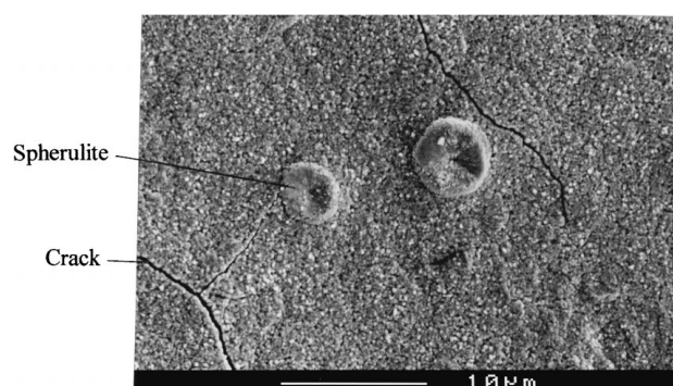
Figure 7 Microphotography of a selenium film iodine post doped at T = 363 K for 6 h with a heating speed of 1 \text{ K min}^{-1} .
